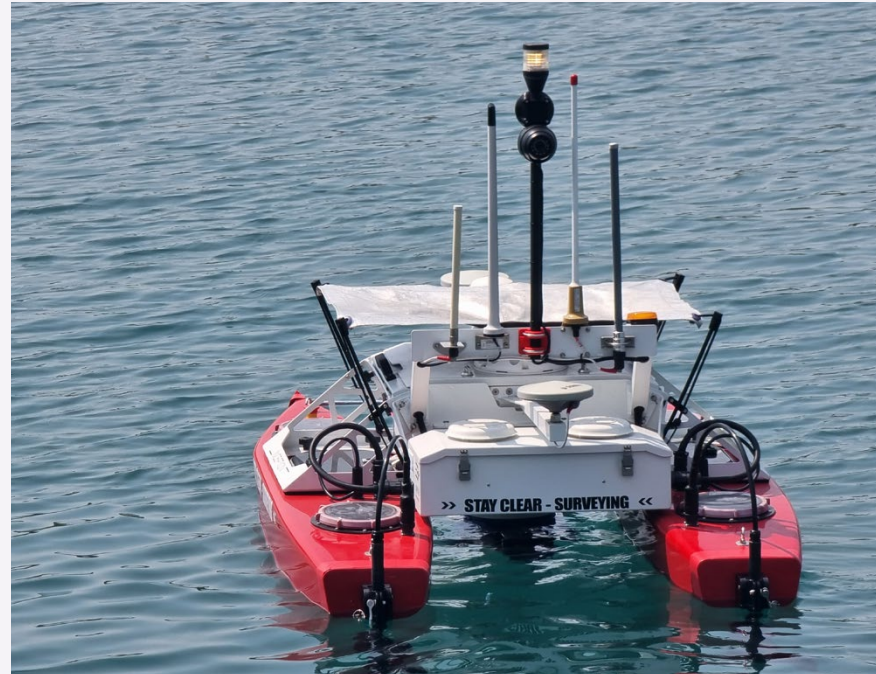
The battery-powered Unmanned Surface Vessel will enhance MPA's capabilities in bathymetric data collection.
