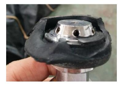
According to passengers' account, after the bottom buoyancy unit was deflated, the floor of the raft began to tear at the side. Under normal operating condition, the raft of the floor was held in placed by both buoyancy units. Therefore, when the bottom unit failed, higher stress was placed on the already stressed floor from passengers' weight that eventually caused the floor to tear at the side.
